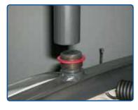
Place the locking ring on the leg stud and screw it on for about 2 turns.
